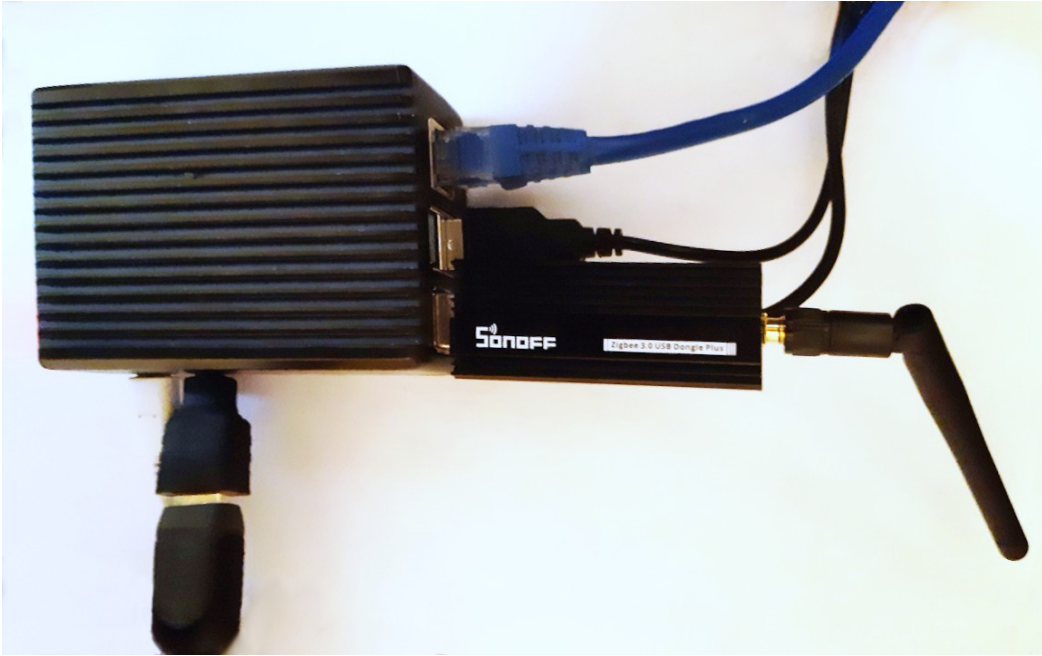
Fig Raspberry Pi with Sonoff Zigbee USB dongle
